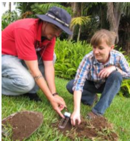
Figure 23. A demonstration of properly burying a soil moisture sensor.
