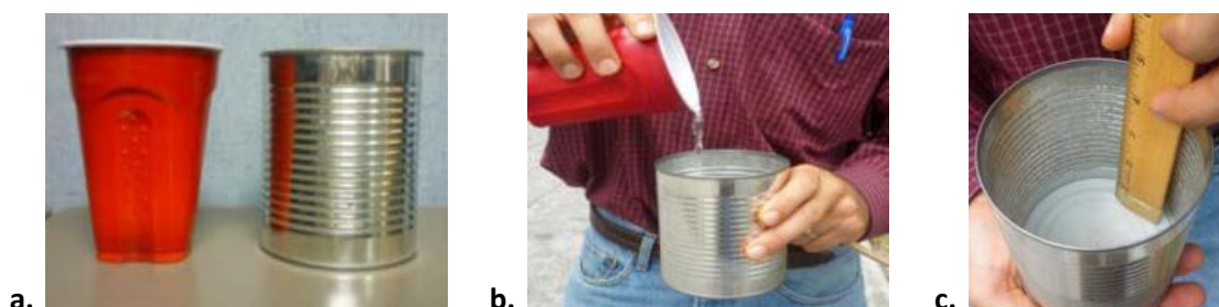
Figure 29. Measuring water collected during a catch-can test.
